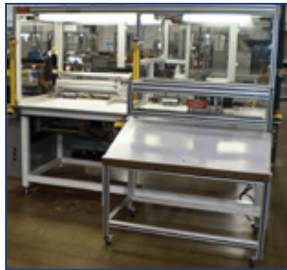
Automatic (left) and semiautomatic (right) RFID tag insertion machines
